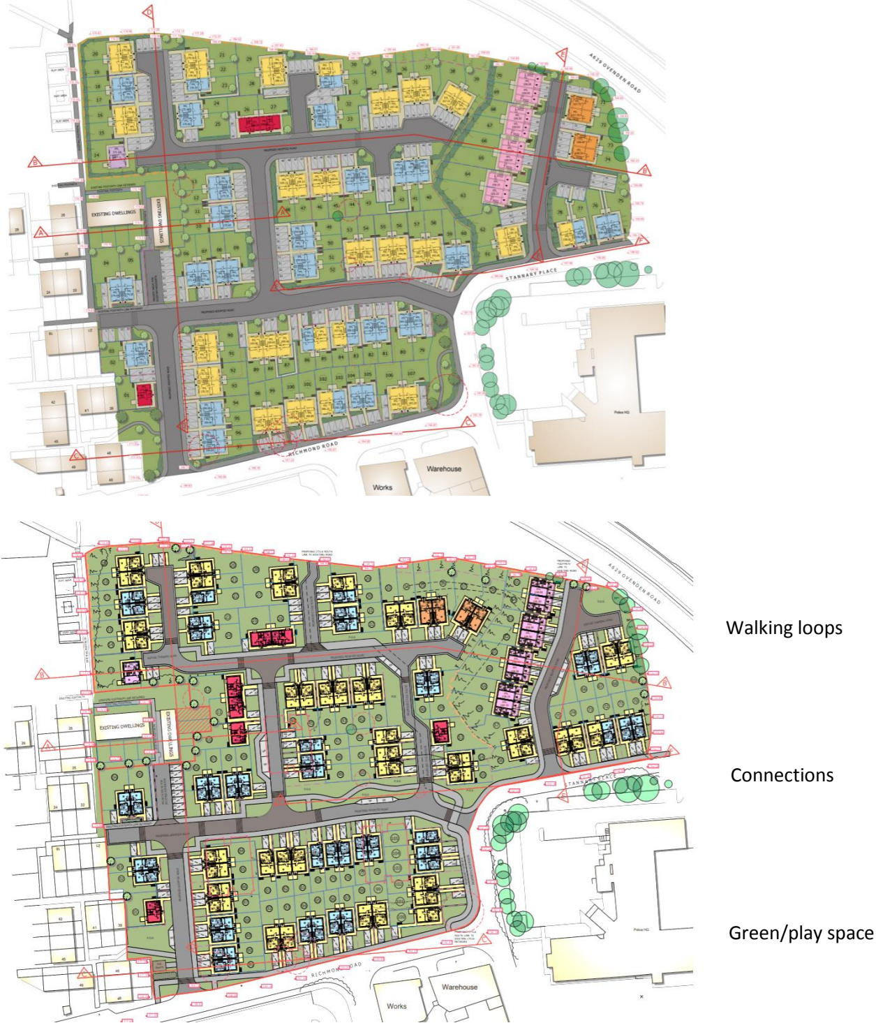
Fig. 4 – Urban design support - example of changes to residential layout to reduce car dominance, improve access to green space and pedestrian/cycle connectivity – the submitted layout (above) and the revised layout (below) which was recently awarded planning permission
